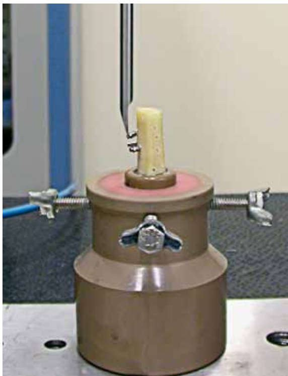
FIGURE 1 - Flexure strength trial using an Emic DL 10.000 universal testing machine.
