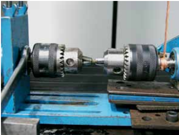
FIGURE 4 - Torsion assay device, performed to determine maximum resistance torque to fracture for the mini-implants, connected to the universal mechanical assay machine with 500N load cell. The right side shaft rotates when the polymer thread is pulled by the assay machine and the left shaft is stationary and holds the mini-implant.
