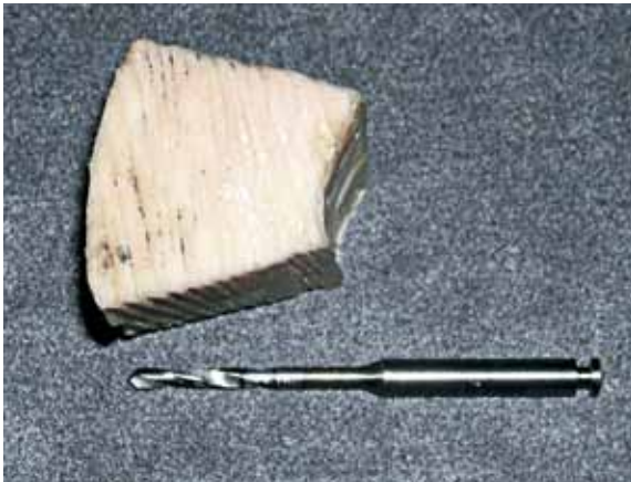
FIGURE 2 - Bovine tibia fragment with 10 mm in width and length and 9 mm in height to allow for complete bur insertion during drilling and also for the evaluated mini-implants.
