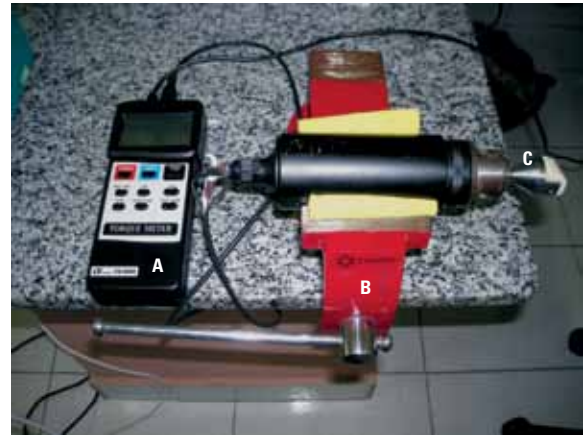
FIGURE 3 - System used to measure mini-implant insertion and removal torques, consisting of a digital torquimeter (a) connected to a bench lathe (b), with a bone specimen, where the mini-implants were inserted, attached by a metallic positioner (c).
