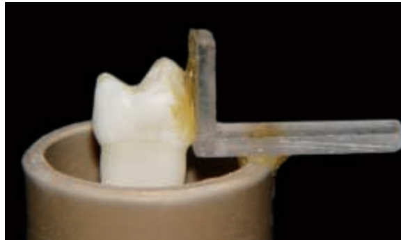
FIGURE 1 - Tooth-square set bonded to PVC tube with sticky wax.
