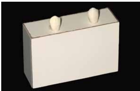
FIGURE 1 - Matrix made of Formica to serve as a replicator. Positioning of the canine crowns that will serve as parameters for the photoelastic model.
