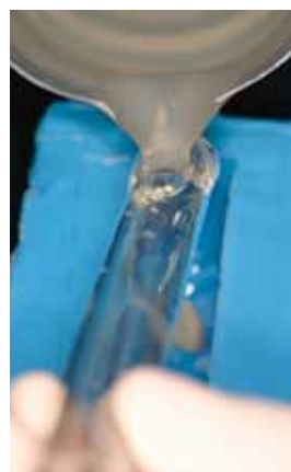
FIGURE 5 - After epoxy resin manipulation, it was poured carefully to avoid incorporation of air bubbles.
