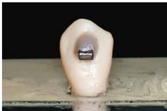
FIGURE 7 - Photoelastic model with 'crossed' tubes in position.
