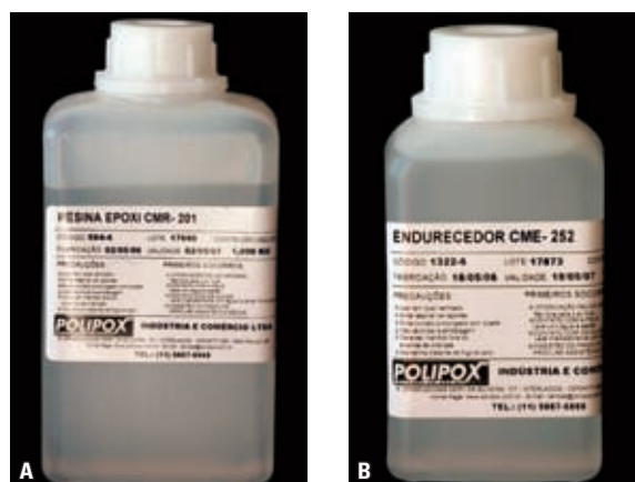
FIGURE 5 - Photoelastic resin: A) COMPONENT "A" EPOXY resin, flexible CMR-201 and B) Component "B" Flexible CME-252 Hardener
