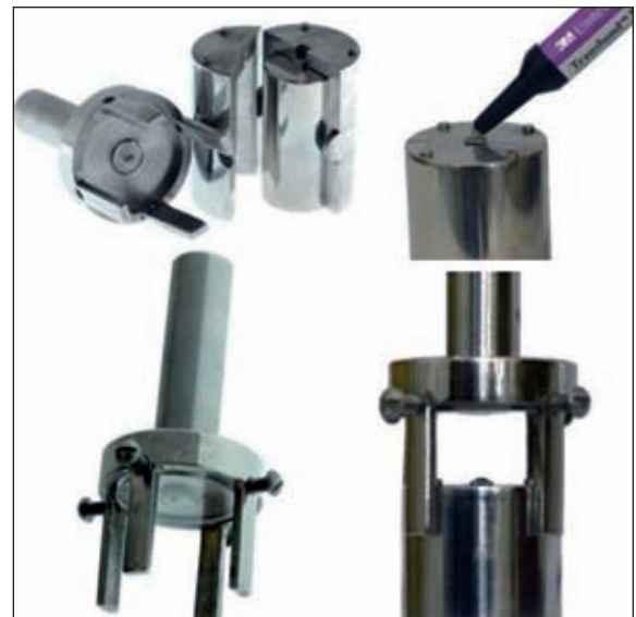
FIGURE 2 - Bonding device used to ensure standardization. Illustration of how the brackets were bonded to the acrylic resin discs.
