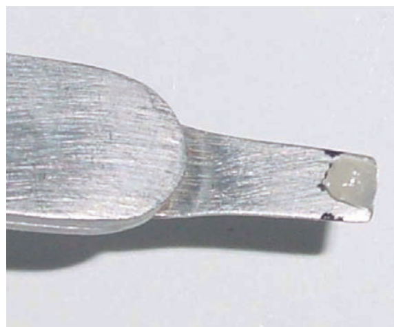
FIGURE 1 - Standardization of additional amount of resin applied to occlusal surfaces of tube/tooth interface in Group 1.
