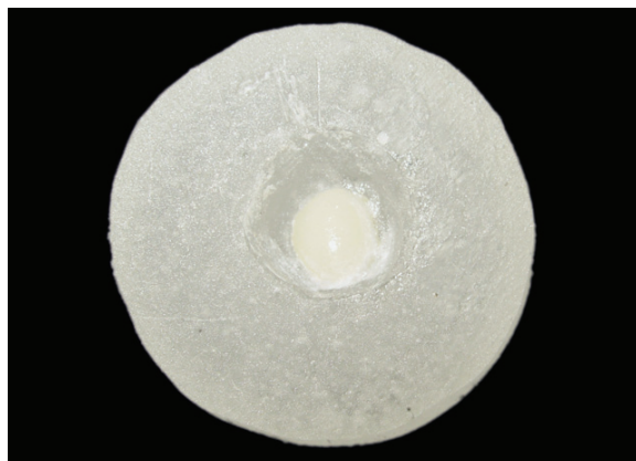
FIGURE 4 - Acrylic cylinder with ceramic specimen adapted with acrylic resin.
