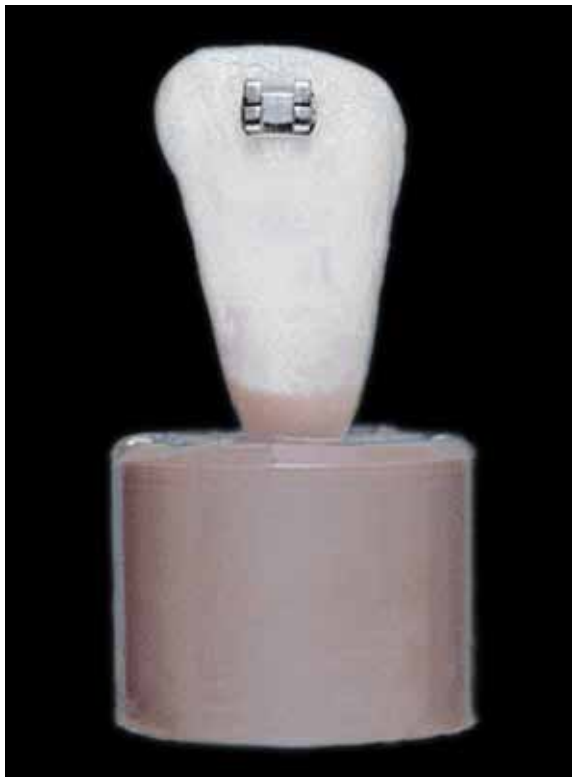
FIGURE 5 - Specimen with bracket bonded to buccal surface.
