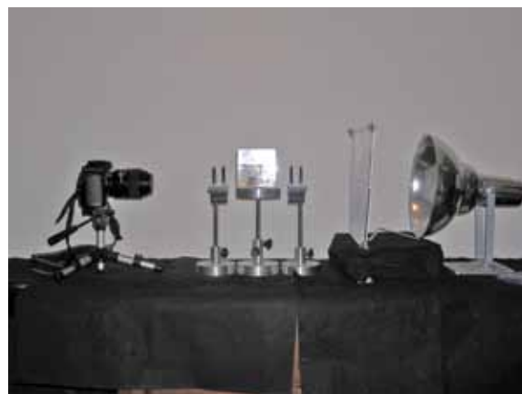
FIGURE 1 - Circular polariscope used in experiment (Eikonal Instrumentos Ópticos, São Paulo, Brazil).
