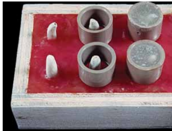
FIGURE 1 - Steps taken to insert bovine teeth in PVC tube.
