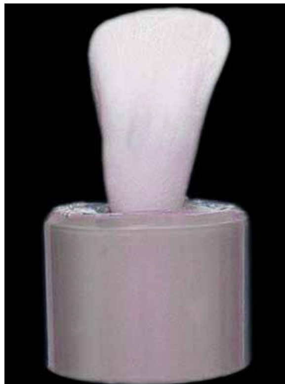
FIGURE 2 - Bovine tooth inserted in PVC tube.
