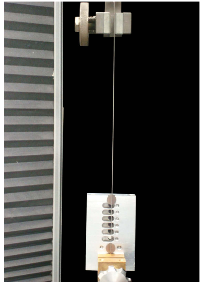
Figure 6 - Device positioning and 0.014-in contour NiTi wire on the Instron machine.
