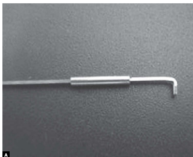
Figure 7 - A) Set comprised of 0.019 x 0.025-in rectangular wire and steel tube; B) set positioned on the vise.
