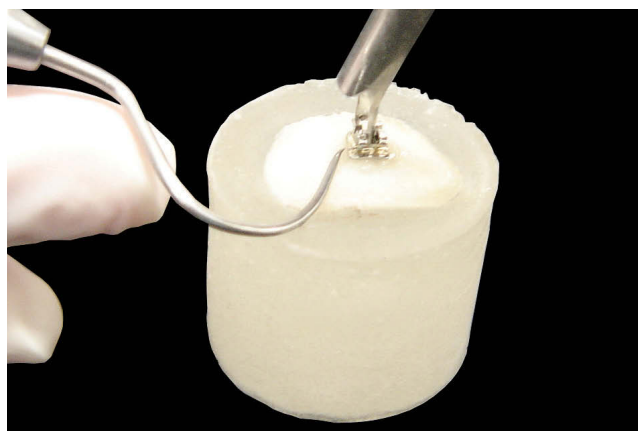
Figure 2 - Bracket being placed under the dynamometer and excesses removed with the probe.
