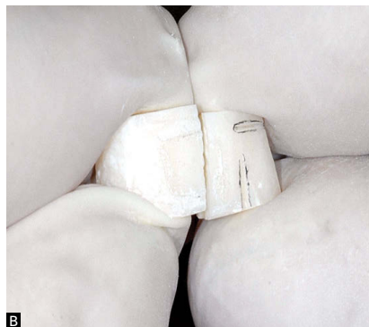
Figure 4 - A) Chisel in position to perform fracture. B) Specimen transversely fractured for SEM assessment.
