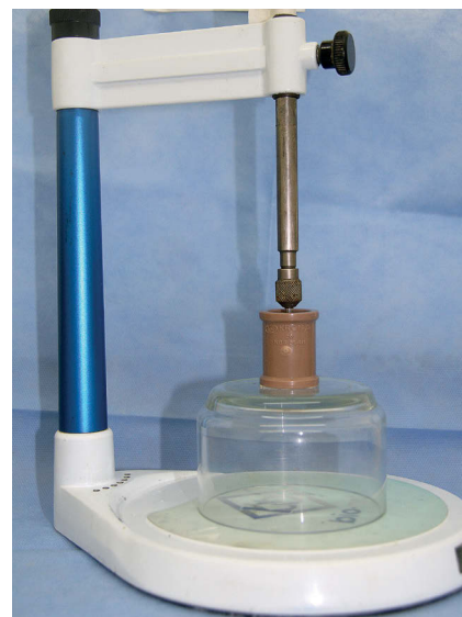
Figure 2 - Implant analog positioned with the aid of a delineator in the PVC pipe.
