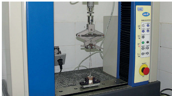
Figure 9 - EMIC machine with the specimen positioned for testing.
