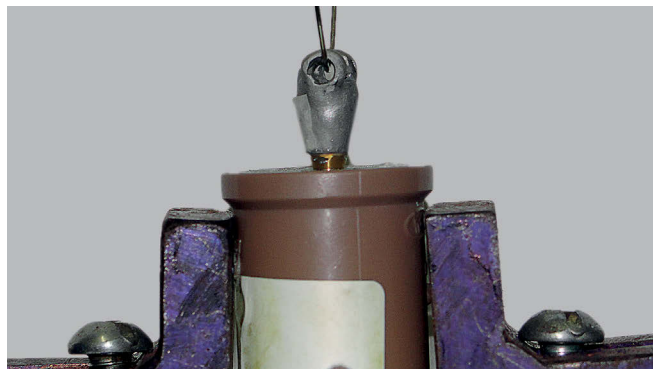
Figure 10 - Approximate view of the specimen positioned in the machine EMIC for testing.
